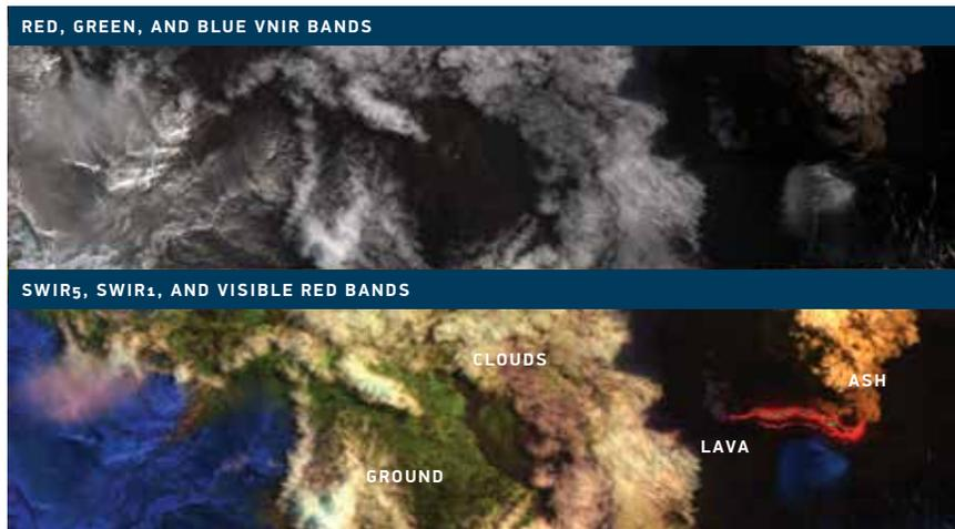
**FIGURE 4.** An image of a volcanic eruption in Iceland shows how snow/ice and clouds appear differently in the SWIR region of the electromagnetic spectrum.
